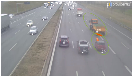
Fig. 1. Live view from one of the measurement points of the Providentia++ test-bed. Sensors (i.e. cameras, radars, LIDARs) observe the highway all the time from which a digital twin of traffic is created providing the tracks of the detected objects (white squares and object IDs). Our approach performs continuous online safety checks based on RSS. Vehicles can receive the check results which show how to escape from potential hazardous situations (sketched overlapping safety envelopes) and get guarded by the system.
